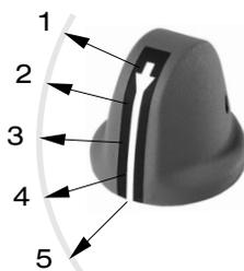
This illustration is the method we utilize in obtaining brightness ratios. A uniformly illuminated source set to a specific brightness in foot lamberts. Photometric measurements are taken at 5 equally spaced locations along the marking, no readings are taken in the area above the metal insert. The average of the measurements (1-5) is the percentage of the brightness of markings to the brightness of the source. This is the brightness ratio, expressed as a decimal.
